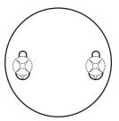
3. Slide the base of the camera downwards so that the screws lock towards the narrow side.
