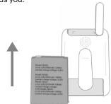
Insert one of the in-box batteries in the bottom of the Baby Unit. The battery should be inserted with the label facing downwards.
