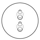
Slide the base of the camera downwards so that the screws lock towards the narrow side.
